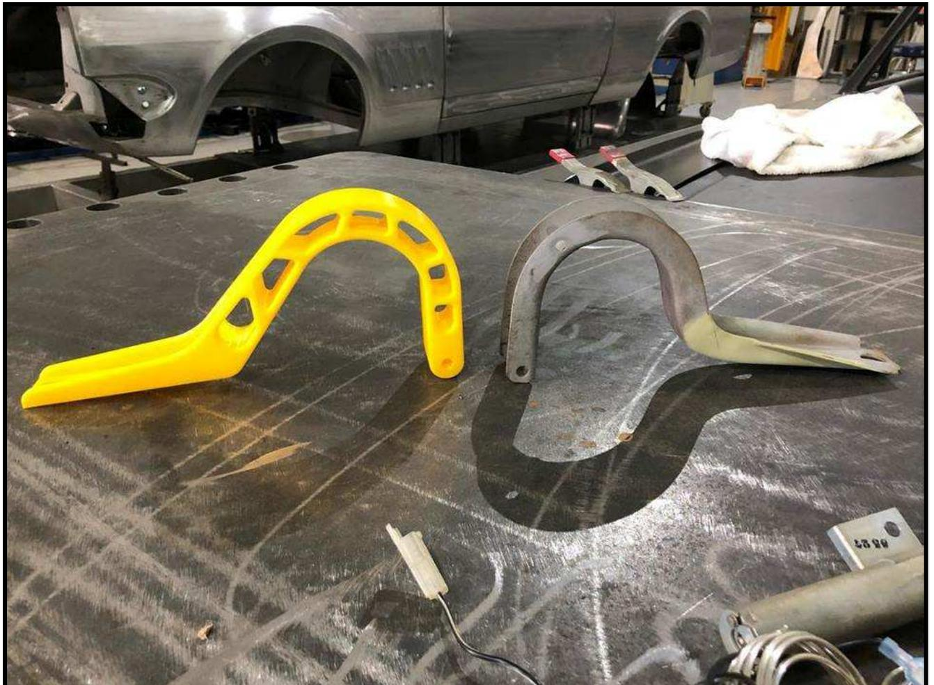
*Test print of a EH Taillight backing being tested for fit prior to machining*
